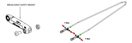
Tighten the bolts of the break-away safety brackets lightly (please refer to the "red arrows" in the above picture).
