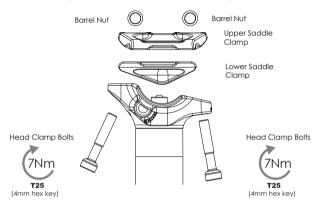
To install the saddle, replace the two saddle head clamp bolts, spherical nuts, upper and lower floating clamp in the order in which they were removed.
