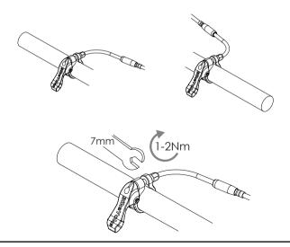
Triggy remote is installed via a snap-on clamp to the handlebar, or optionally via I-Spec adapters.
