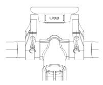
Open the clamp on the D-pad and place it in the correct position, Using 1 X M3\*12 screw tighten the D-pad onto the handlebar. Torque requirement: 1N.m.
