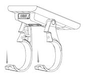
Now place the display on to the handlebar in the correct position. Now with 2 X M3\*12 screws tighten the display into position. Torque requirement: 1N.m.
