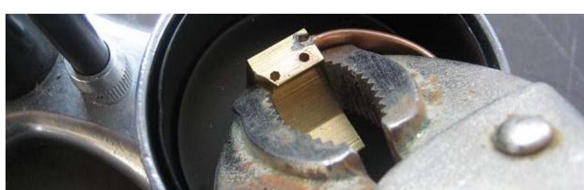
**Step 4 - Replace gauge sealing O-ring:**
