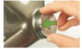
If the gauge only fits one side of the frame or is only slides in partially, it is a **NO-GO. Do not force the gauge into the frame.**
