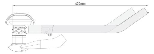
Minimum insertion - the extension must completely fill the window in the bracket.
